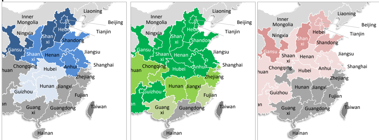
Figure 8: Payback period for ASHP versus resistance heating, gas heating, and coal heating by province
