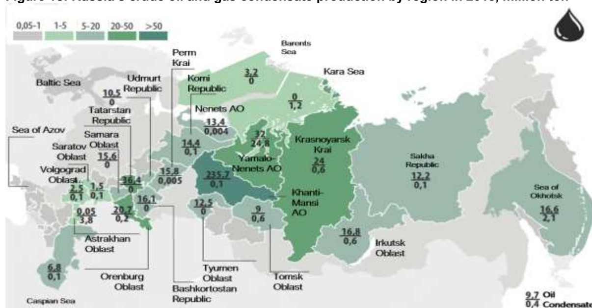
Figure 18: Russia’s crude oil and gas condensate production by region in 2018, million ton
