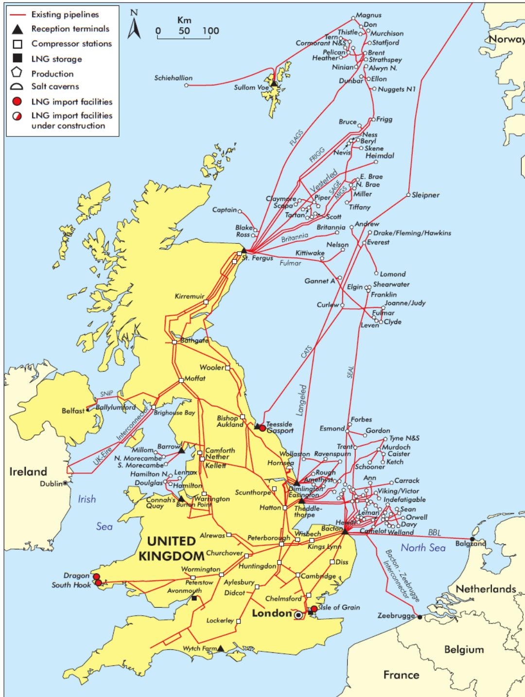
Figure 19: Main UK Offshore and Onshore Gas Infrastructure
