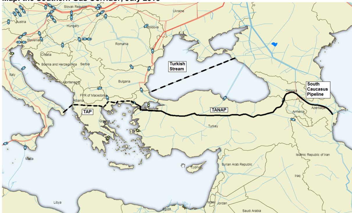
Key. New pipelines to south-eastern Europe: black (completed) and black broken lines (projected). Other gas pipelines: red (large diameter) and blue (other).
