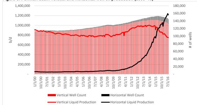
Figure 6: Permian basin vertical and horizontal well oil production (2000–16)
