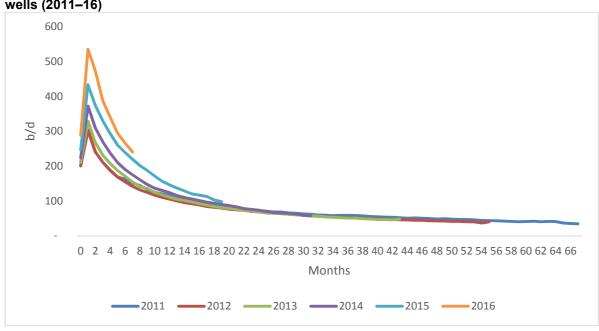
Figure 2: Aggregated oil decline curve for horizontal Permian, Williston, and Powder River wells (2011–16)
